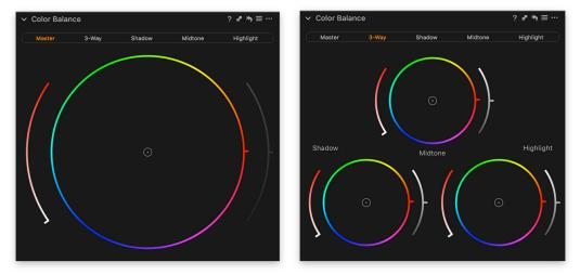
Use the Master Color Balance tool to imbue the desired color balance on the overall image. If needed, use the 3-Way Color Balance tool to tweak the color balance of just highlights, mid-tones, and shadows.
