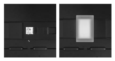
Remove the film and the film carrier together from the positioning stage. Replace the carrier with a piece of matte, translucent Plexiglas seated in the same plane of focus as the film.
