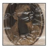
**Delamination or Channeling** The base of acetate films can shrink over time, causing the emulsion to bunch up in a way that creates visible channels.
