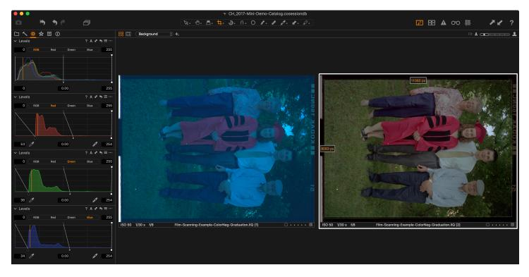
In the case that many similar frames are captured at the same time it may be more consistent and accurate to identify the frame that contains the most neutral shadow and highlight subject matter, auto adjust to that frame, and then copy-apply those adjustments to the other frames.
