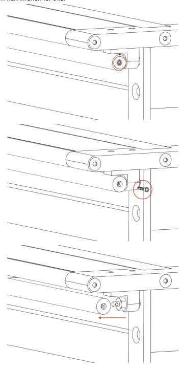
2. Unscrew the latch bolt by using an adjustable wrench or pliers
