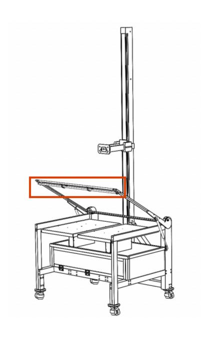
The DT Versa features an ergonomic glass top latch that allows for the lift and locking of the glass platen. This component has been carefully selected and tested for maximum durability and reliability. However, as with any moving part, it will eventually wear and require replacement.
