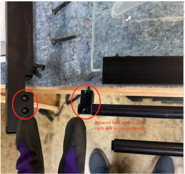
4a - In order to remove the round handle, remove both screws using a 1/8th T-wrench on each side. Do not lose the thin spacer in between.
