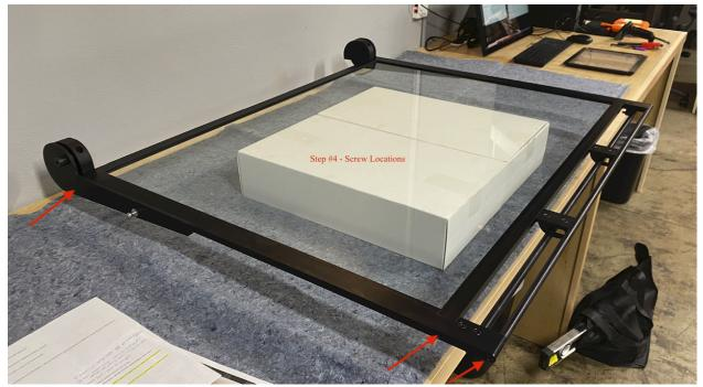
4 - Remove the 3 screws on the side of the frame which attach the cross pieces (1 threads into the round handle, 1 threads into the front cross beam, 1 threads into the rear cross beam), using a 1/8th T-wrench. Repeat the process on the opposing side of the frame. See reference image above.
