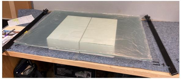
7 - Realign the frame with newly attached glass to the Versa table. Attach the (4) shoulder hinges followed by locking down the (2) air springs on each side.
