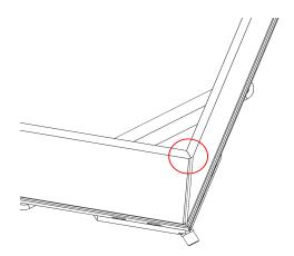
10. Insert both panes of glass into one of the V-brackets.
