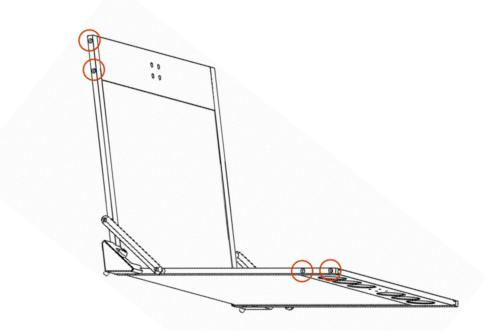
5. Remove the side panel (A) by removing the opposing 2 bolts (B)
