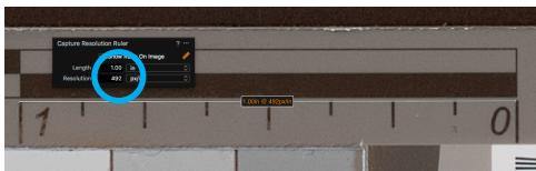
With the carriage at this position, enter live view, focus the camera, take a picture, and record the resolution (PPI) using the “Capture Resolution Ruler.”
